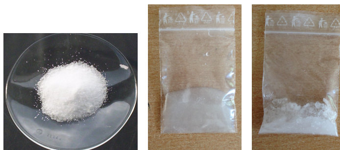
Figure 2. Glauber’s salt in anhydrous and decahydrate (melted and solid) form
