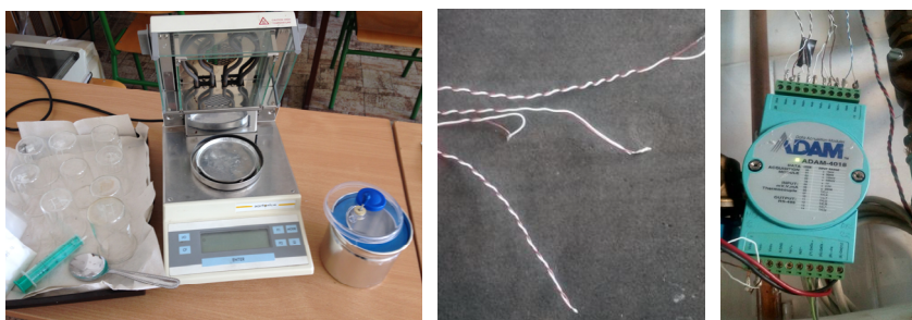
Figure 3. Used equipment: scale, calorimeter, thermocouples, ADAM module
