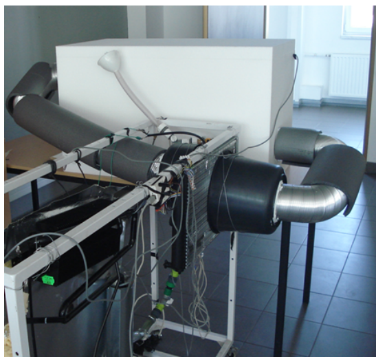
Figure 5. Engine's heat exchanger in the experimental unit (Department of Physics and Process Control, SZIU)
